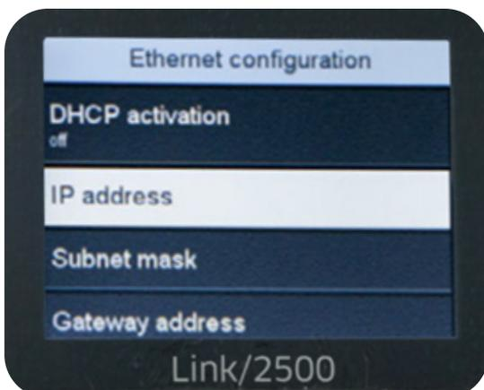
3C) Select “IP address”. Enter the static IP assigned to the device then press the green “Enter” key.
