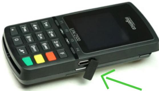
2A) Lift the flap on the side of the Link/2500 covering the charging port.
